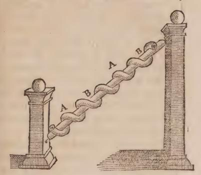
Where you see there is a Cylinder AA, and a spirall cavity or pipe twining about it, according to equall revolutions BB. The axis and centers of its motions are at the points CD, upon which being turned, it will so happen that the same part of the pipe which was now lowermost, will presently become higher, so that the water does ascend by descending; ascending in comparison to the whole instrument, and descending in respect
